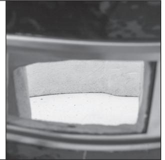
**15** Insert the charcoal grate in the bottom of the fire box, then add the cooking grate as shown in the photo.
